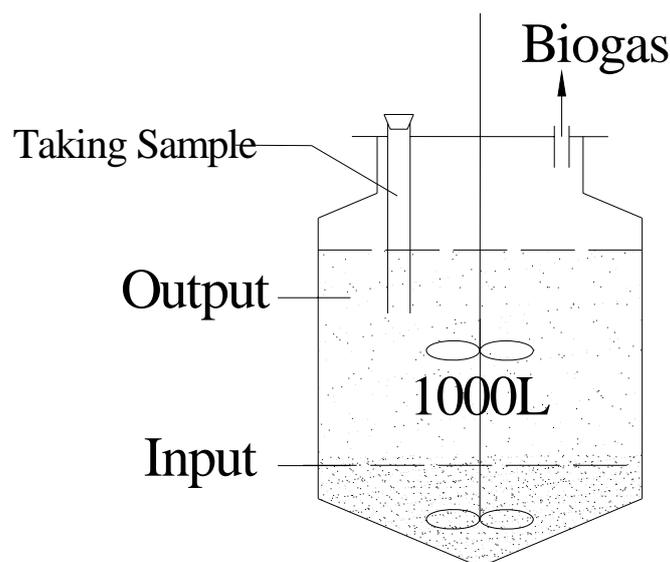
Figure 2: Sketch of a biogas-digester used in the field experiment
