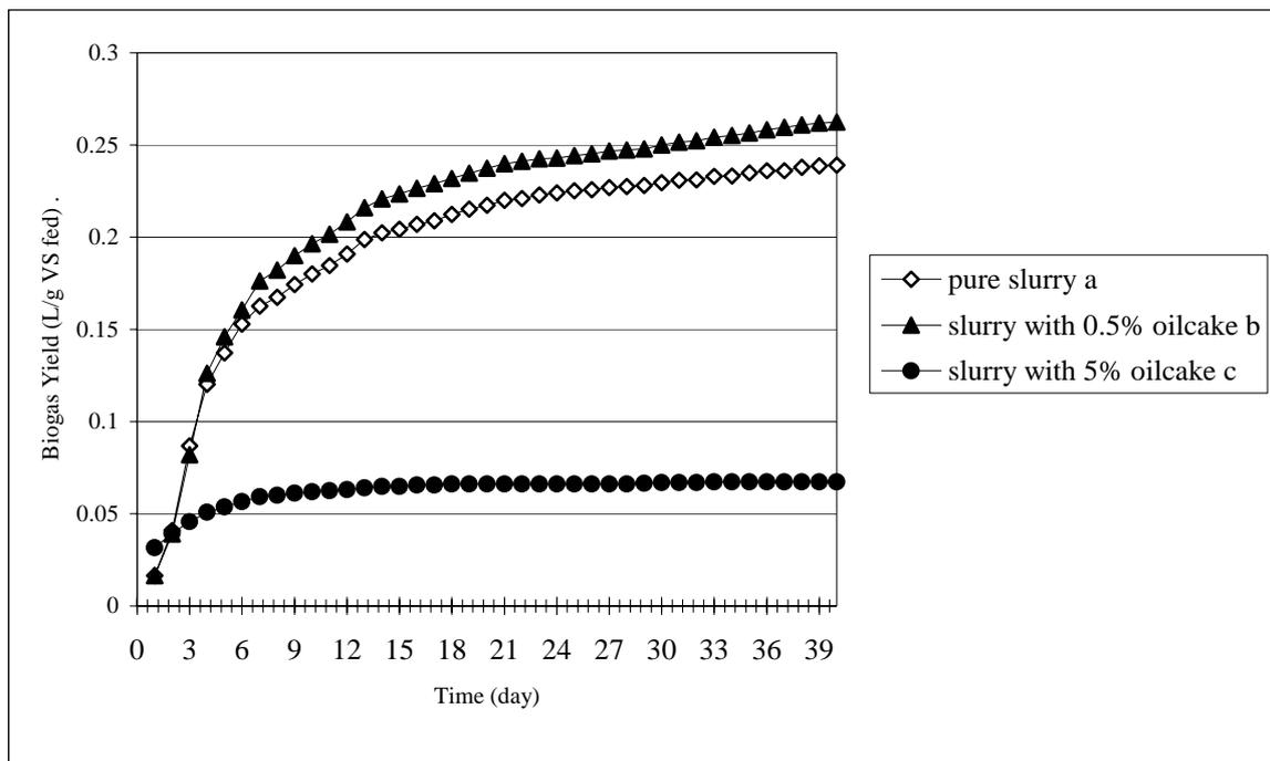
**Figure 11: Mean cumulative biogas production for lab-scale fermentation**
