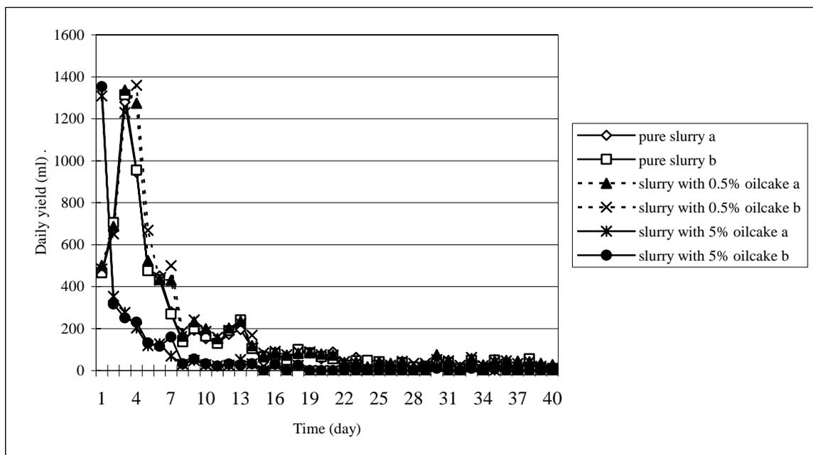
Figure 10: Daily biogas production for lab-scale fermentation
